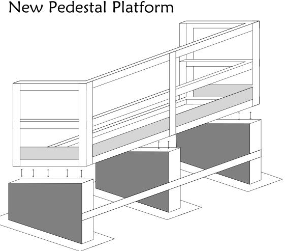
Ideal for shingled, metal seam or PDM pitched roofs. They offer great support as well as easy installation With our pedestal platforms there is no need for expensive flashing boots. Pedestals are constructed of 16g stainless steel and welded liquid tightat all seams.
