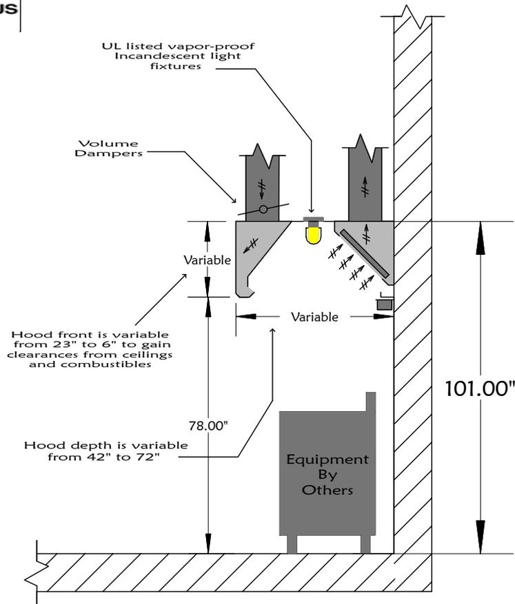
Lowering the front of the hood, lowers the top in order to keep the front at 78" from the floor. Where the top of the hood is at 101" on a standard canopy. The top of a 6" low profile is at 84". Thereby increasing the distance from a ceiling containing any combustibles.
